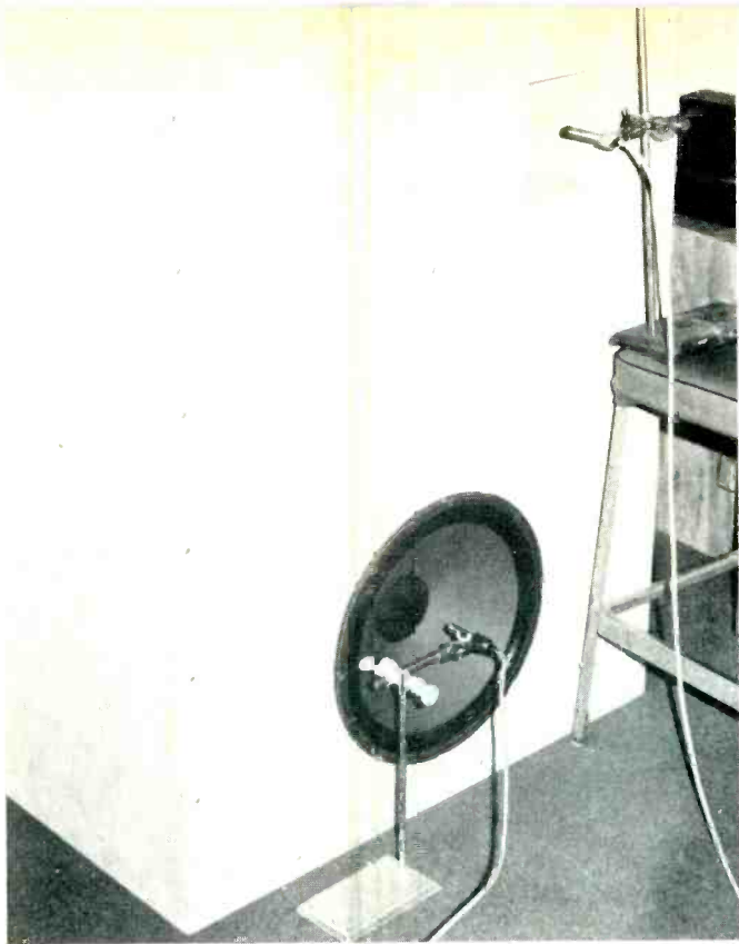
Fig. 9—Microphone placement for Keele's method of measuring nearfield sound pressure.
