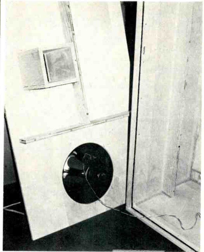
Fig. 3—Installation of the front panel gasket. Note the damping material, braces, and vent.
